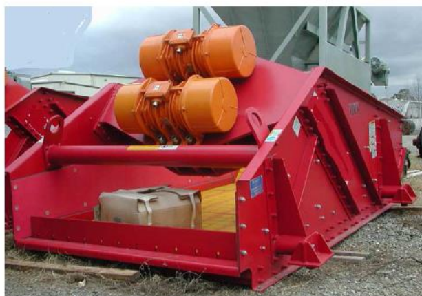
Figure 6 Vibrating dewatering screen
